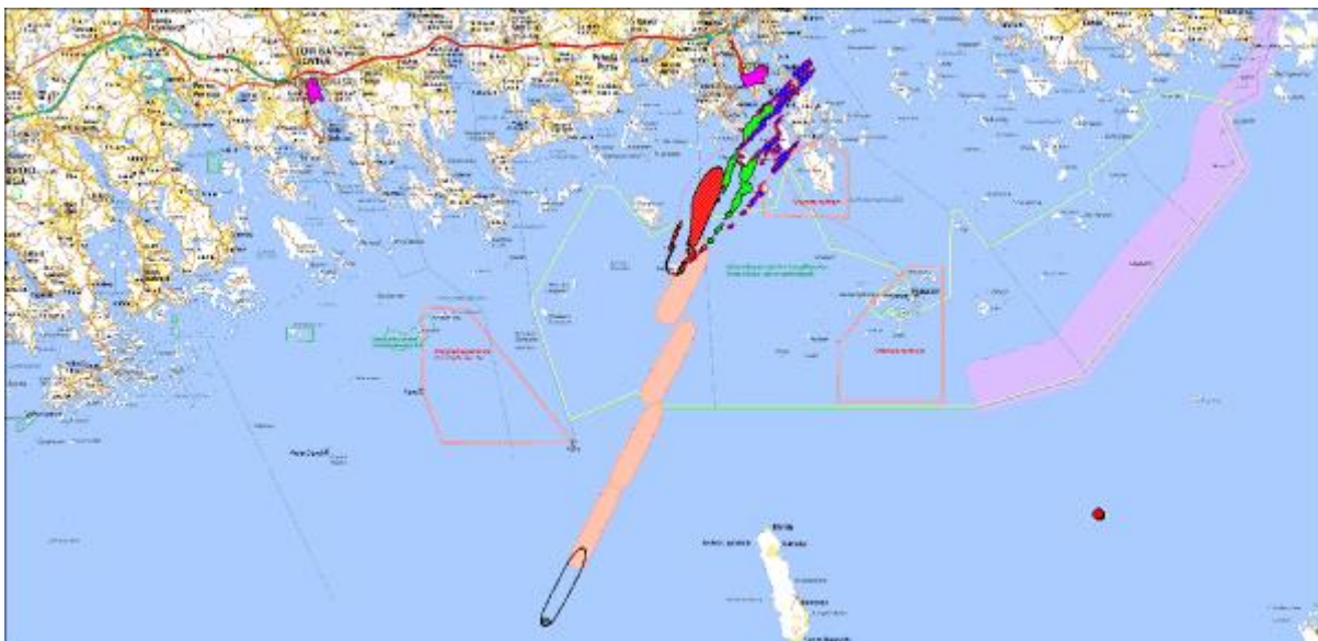
Map of the drifting scenario. The map shows the calculated slick positions in 6 hour time steps. The red area in the map shows the slick position at the start of the exercise, green and blue areas indicate the slick drift during the exercise.
